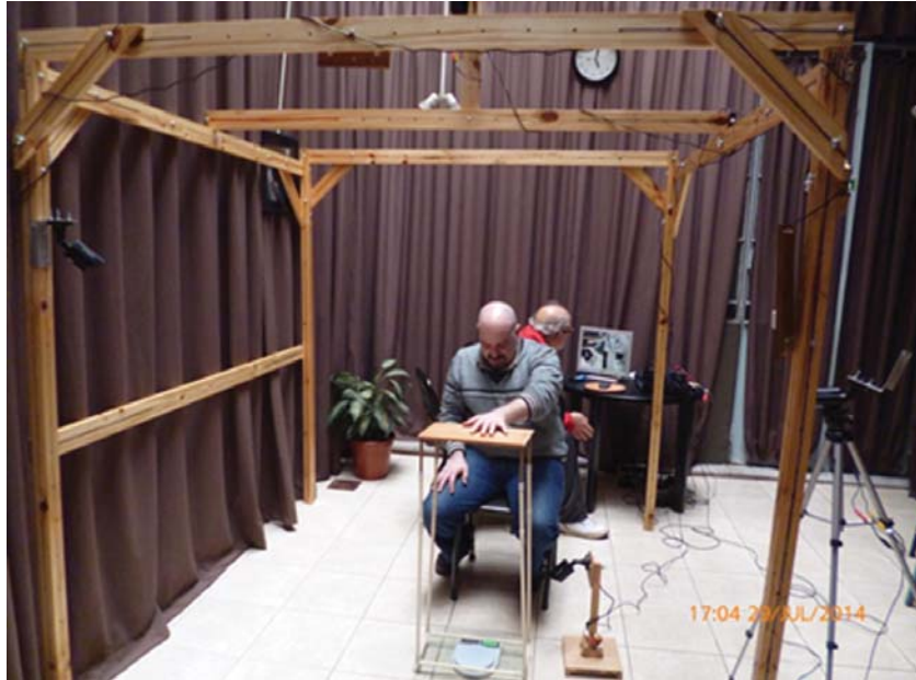
Photo 1. Panoramic view of the PK laboratory showing the wooden frame for mounting video cameras, with Ariel Farias at the center. There are cameras in the left column, above Ariel and near his left leg. To the right, there is another camera mounted in a tripod. At the right column, the microphone is mounted. Behind Ariel, one of the investigators is monitoring the work through the screen of the DVR. The photo shows Ariel trying to raise a little wooden table (weighing less than 400 g), mounted on a plastic structure, over a piece of flat glass, this last supported by a scale. This setup allowed Ariel to experiment with variations of the main phenomena, and to get feedback from the scale's display variations, during concentration and work.
