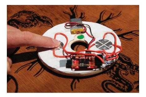
Figure 3. Planchette with additional sensors.
