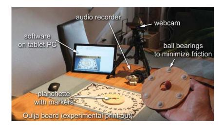
Figure 1. Experimental setup.
