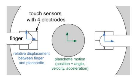
Figure 4. Principle of capacitive sensors.
