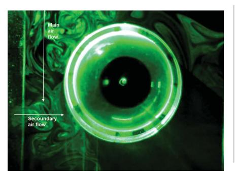
Figure R1. Combining vertical and horizontal air flows to set the HM in motion.
