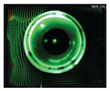
Figure R2. Vector-field representation of the mean air flow speed around the mobile.
