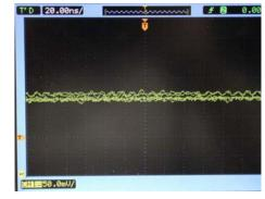
Figure 18. Noise produced by the DAC and power supply. CY8C5588AXI 060 with internal amplifiers, DAC, and ADC. Accuracy of measurement is about 3%. The system is powered at 5 V through a USB interface from a laptop. The noise from the DAC and power supply is shown in Figure 18 and is in the range  $\pm 10$  mV, about 0.3% of the voltage generated. To reduce the level of noise, a software filter averages values
