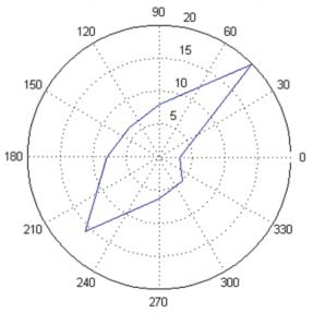
Figure 2. Polar plots of the signal strength when ball antennae are used for both transmit and receive functions, both without (above) and with (below) the polarizers in place. The angle of zero represents the frontal face of the Tx ball antenna. The main effect of the polarizers was to shift the angle at which the signal is strongest by  $\pi/2$ .
