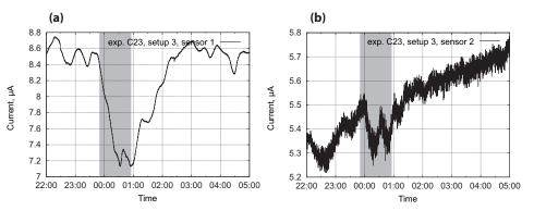
Figure 11. Experiment C23 with setup 3 of the detector and the LED generator, d = 15 cm, LED generator using the first waveform. (Gray area) The LED generator was switched on between 23:47 and 00:57.
