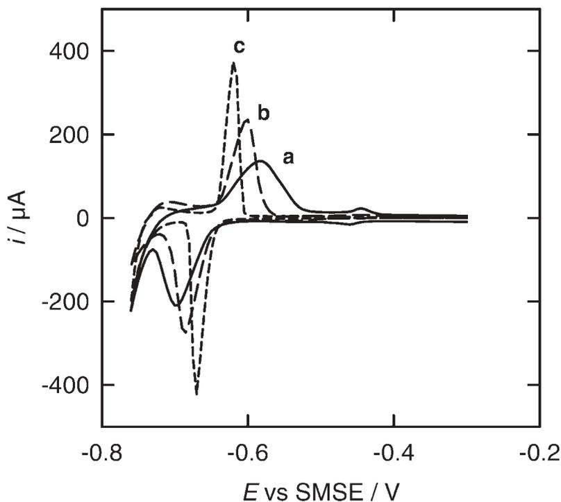
Fig. 1. Set of cyclic voltammograms of H<sub>1</sub>-e Pd (200 nm thick, deposition charge 3.5 mC, deposited from the Brij<sup>®</sup>56 plating bath) deposited on a gold disc electrode (area 0.0079 cm<sup>2</sup>) recorded at 10 mV/s in 1 M H<sub>2</sub>SO<sub>4</sub> (a) without crystal violet, (b) in the presence of 0.5 mM, and (c) 1 mM crystal violet.
