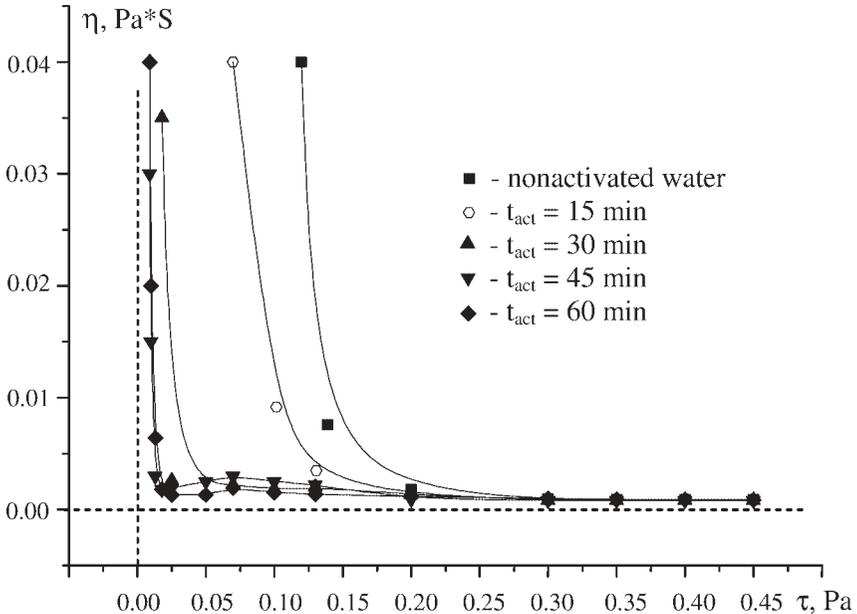
Fig. 2. Viscosity  $\eta$  of nonactivated water and four fractions of activated water in the region of small shear stresses  $\tau$  at a temperature of 36.6°C.
