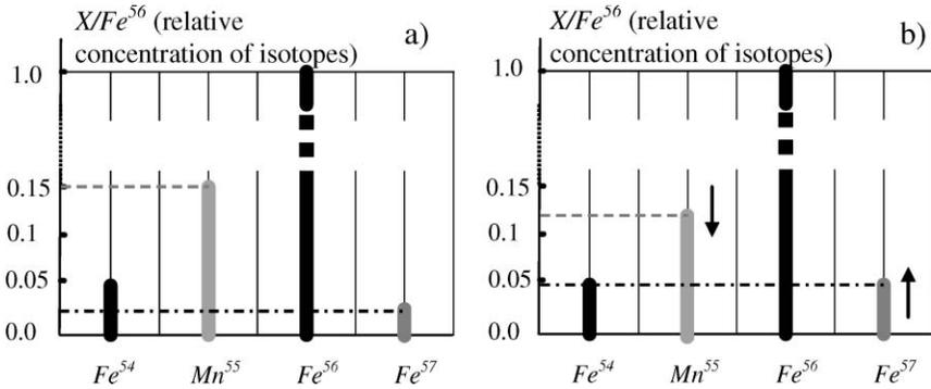
Fig. 3. Mass-spectra of iron-region of microbiological associations (dried biological substances) that were grown in control nutrient medium with  $H_2O$  and  $Mn^{55}$  (case a) and in experimental nutrient medium with  $D_2O$  and the same quantity of  $Mn^{55}$  isotope (case b). The process of increasing ( $\uparrow$ ) of concentration of  $Fe^{57}$  isotope is accompanied by decreasing ( $\downarrow$ ) of concentration of  $Mn^{55}$  isotope. Here  $X = Fe^{54}, Mn^{55}, Fe^{57}$ .
