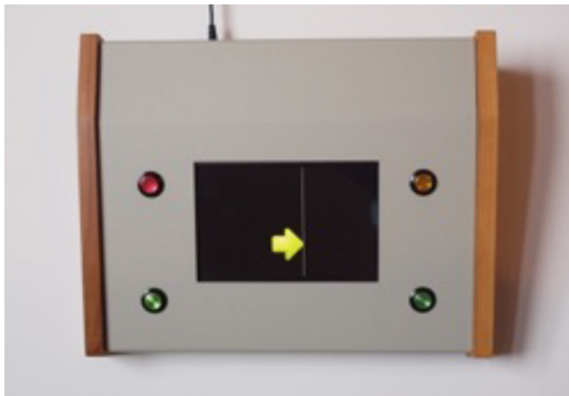
Figure 1. The experimental apparatus. The video screen shows an arrow the direction of motion of which was to be 'influenced' by the participant, while being driven by true random events.
