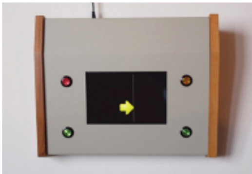
Figure 1. The experimental apparatus. The video screen shows an arrow whose direction of motion was to be ‘influenced’ by the participant, while being driven by true random events.
