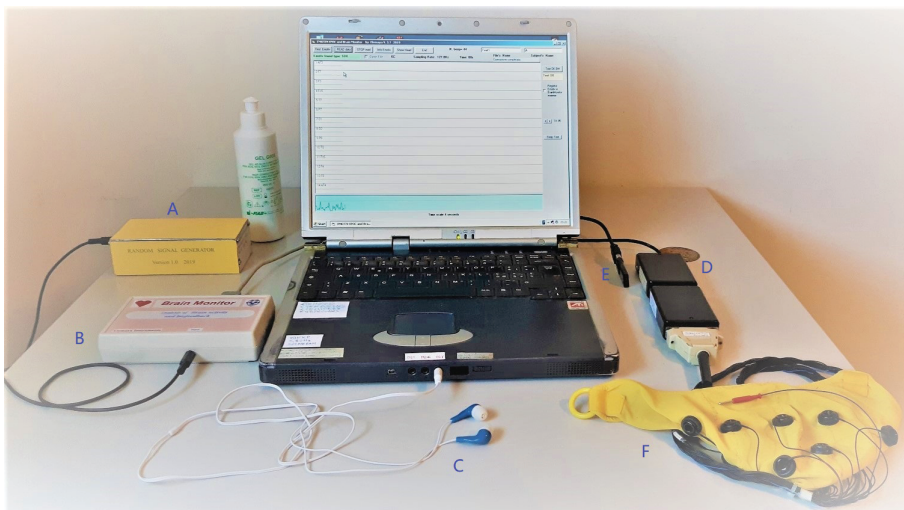
Figure 2. Hardware used in this study. Computer + A = RSG, B = amplifier and analog/digital converter, C = headphones, D = modified Emotiv EPOC, E = 2.4 GHz USB receiver, F = EEG headset.
