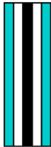
Figure 2. Side view of the separating wall at one of the 5 “interaction zones.” Glass (green), paper sheet facing either the left or right side (hatched white), metal wall (black), and glass (green). A thermal insulating layer may be added if necessary.
