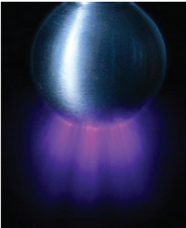
Figure 2. Direct-current corona discharge of negative polarity on a spherical surface, showing a stage with an amalgam of moving streamers blurring into a broad glow in blue to purple colours (from Riba et al., 2018, p. 10, fig. 4b).
