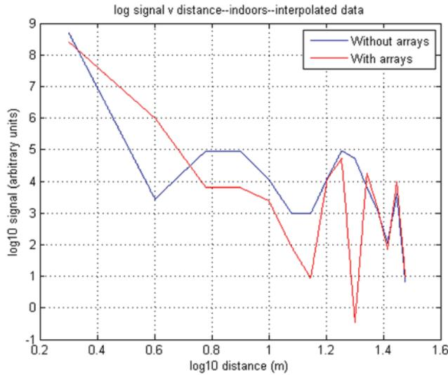
**Figure 3. Results of an experiment conducted indoors, in an east–west oriented hallway of length 30 m.** We present the signal intensity recorded both without the polarizer-analyzer arrays (blue), and with them in place (red). With a few exceptions, most notably the data point at a distance of 20 m, the shapes of the curves are similar.
