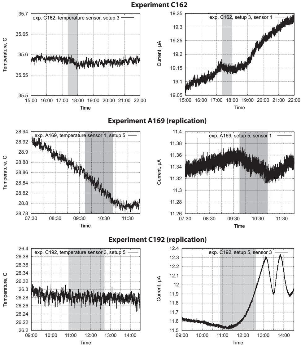
**Figure 7. Impact of temperature variation on the sensors in laboratory B.**
