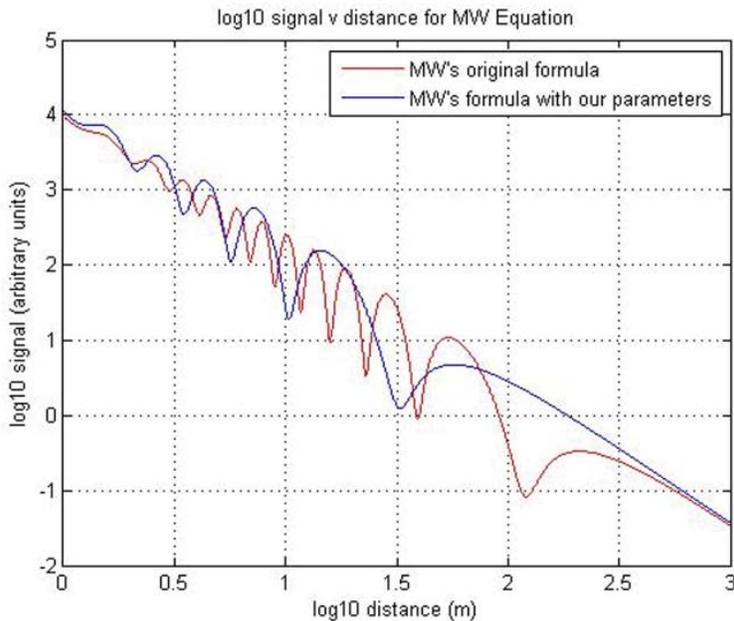
**Figure 1.** The graphs were generated numerically using MW's signal equation, using MW's parameters (red), and adjusted for our actual input values (blue). The only changes were a reduced height for the transmitter and receiver, and a slightly higher frequency. We extended the study down to a minimum separation of 1 m, whereas MW used 10 m.
