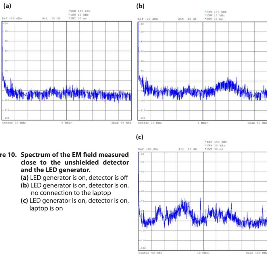
**Figure 10. Spectrum of the EM field measured close to the unshielded detector and the LED generator.**
