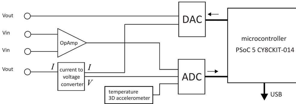
**Figure 17. Structural scheme of the experiment setup.**
