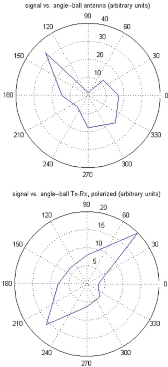
**Figure 2.** Polar plots of the signal strength when ball antennae are used for both transmit and receive functions, both without (above) and with (below) the polarizers in place. The angle of zero represents the frontal face of the Tx ball antenna. The main effect of the polarizers was to shift the angle at which the signal is strongest by  $\pi/2$ .
