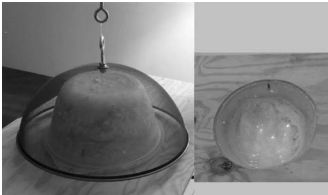
Figure 7. Left: The “Helmet” under the suspended pendulum. Right: The “Helmet” seen from below. Construction of the “Helmet”: Inner layer is a rigid plastic hemisphere with a 20.3 cm inside diameter, ~0.3 cm thick; Outer layer is a soft plastic food container with a 23.2 cm inside diameter at the rim. Between the two layers is a mixture of Dow Chemical “Great Stuff” insulating foam and DAP Products multi-purpose foam sealant.
