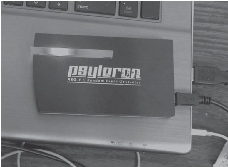
Figure 2. Random event generator (REG); A Psyleron REG-1 device used throughout the following experiments.
