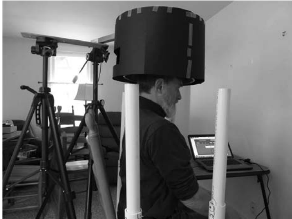
Figure 5. The experimental setup with the “Windshield,” a cylinder of construction paper and foamboard. The pendulum is free to oscillate inside it.
