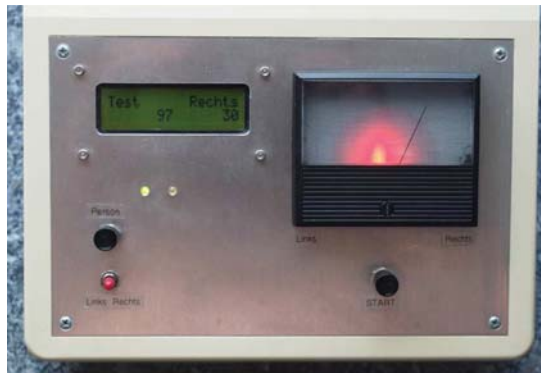
Figure 1. The experimental device, photographed in a state with active display, simulating a real data-taking run. The needle (upper right) has moved to the right-hand side during this run, as a result of the random walk, accumulating the binary random generator output. The alphanumeric display on the upper left side of the image shows the name of the participant (here Test), the chosen intention (here in German Rechts for right), the actual accumulated random generator bits as deviation from equal distribution (here 97), and the remaining seconds for the actual run (30).
