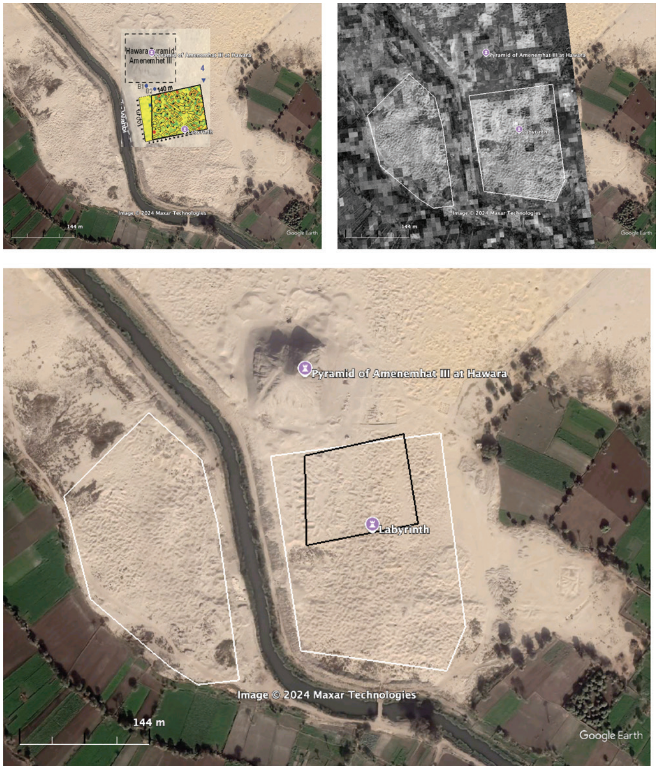
Figure 11. Khalil et al. (2010) in situ VLF-EM Survey (Top Left) and Uncorrelated SAR-Visible Returns from Figure 9 (top right). The uncorrelated SAR-visible returns occur over the same area (bottom) as the VLF-EM survey. (Google Earth).
